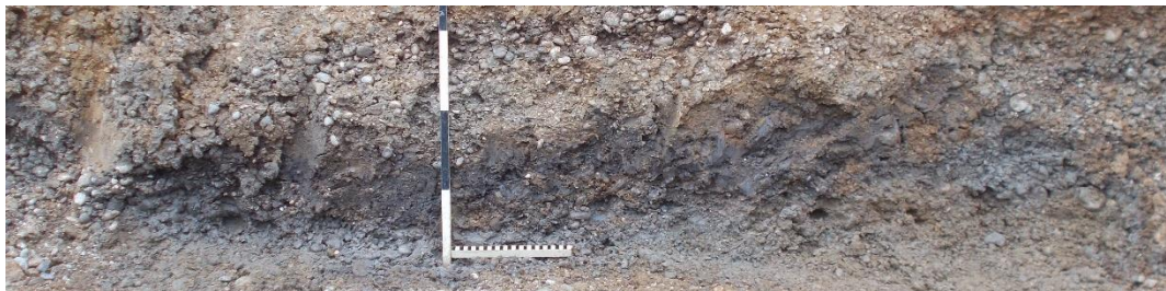
Pl. 6: Clay Block [30] Within [13], Cell 3, West Exposure, Looking South (Vertical Scale in 20 cm Divisions)
